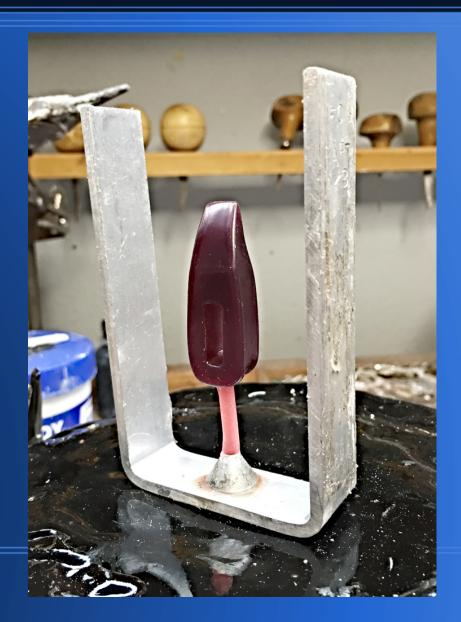
Seal the sideplates to the mold frame with hot glue
