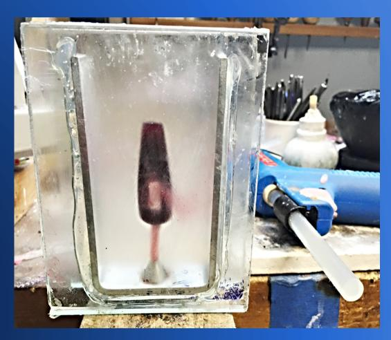
Mix and vacuum the mold compound following the directions, pour and vacuum again, allow to cure.
