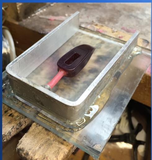
Seal the sideplates to the mold frame with
